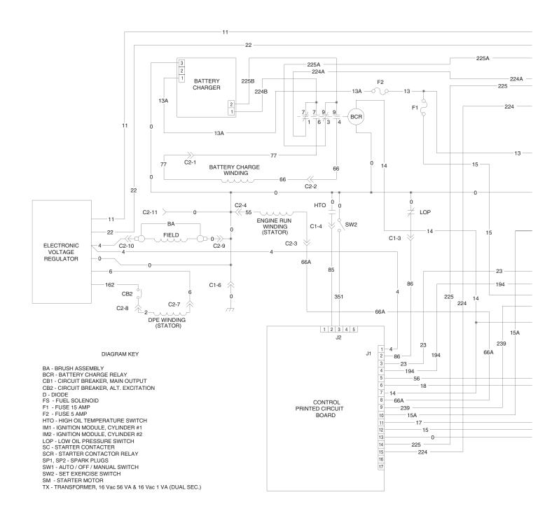
Air-cooled 8.5 kW Generator Electrical Schematic - Drawing No. 0D8501-B
